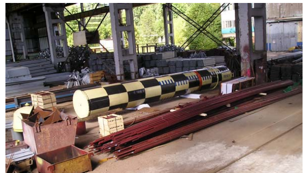
Fig. 6. Hull of FWEPS demonstrational module under manufacturing.
